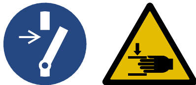
66947 – Inspection cover/inspection door: “Disconnect completely before working”, “Warning of risk of crushing”
